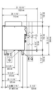
EQ = Equipotential screwG = Gas connection
